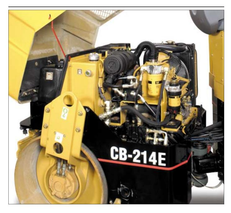
Fiberglass engine enclosure pivots upward and locks open with a prop rod.
