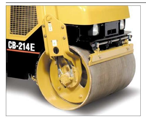
Specially designed drum edges help eliminate marks on deep lifts or when turning. Note: The CB-214E and CB-224E can be equipped with optional Non-Machined Drum Edges that have a square profile instead of the standard design.
