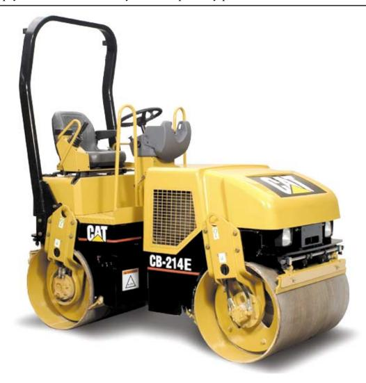
The CB-214E, CB-224E and CB-225E are versatile machines that can be used as the only compactor on small sized jobs or on larger jobs as a support roller for high-production compactors. As a support roller, they work well for turning lanes, cross-overs, shoulders and other similar sized jobs.
